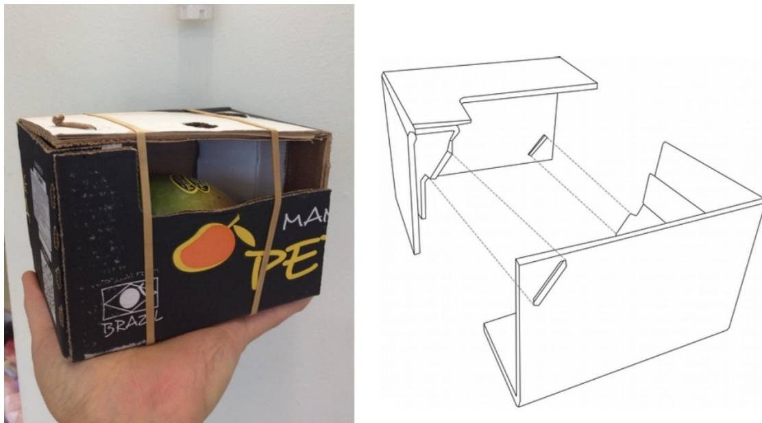
Figure 3. Design of a “Mango Equivalent Unit” (MEU).
