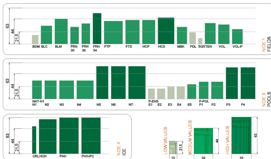
Figure 7. Study of the special height needs of sport courts according to the NIDE regulations.
