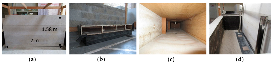
Figure 6. Experimental laboratory set-up built to test the efficiency of a wall-base ventilation channel for drying flooded walls: (a) dimensions of the limestone walls; (b) ventilation channel with a waterproof membrane on the outside; (c) interior of the ventilation channel; (d) final experimental configuration.
