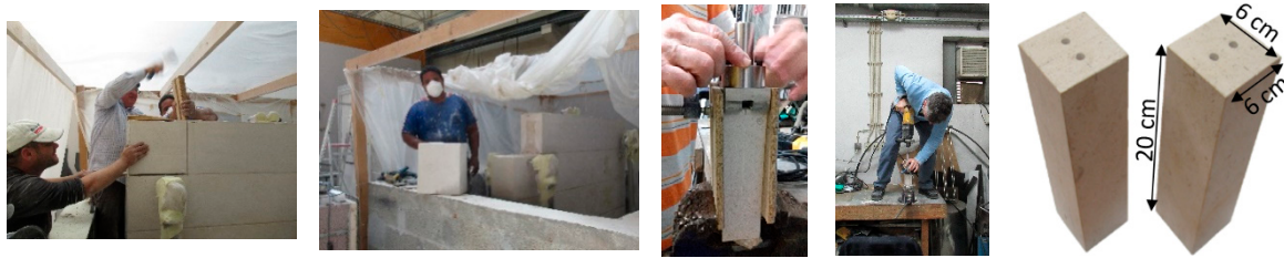
Figure 11. Preparation of the limestone samples for the calibration process through the gravimetric method.
