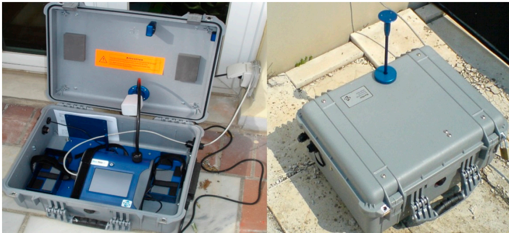
Figure 1. PM 10 monitoring instrument (Dusttrak 8530) placed inside its environmental enclosure.
