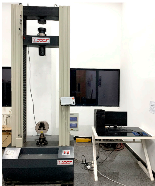
Figure 3. WDW-300 microcomputer controlled electronic universal testing machine.
