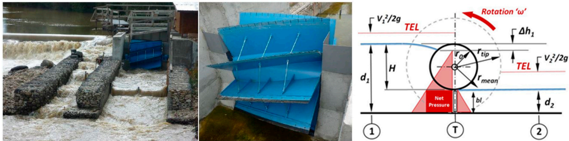
Figure 45. Hydrostatic Pressure Machine (HPM) under real field trial, developed by the HYLOW project, Bulgaria (reprinted from [61]), and 2D scheme of an HPM under nominal operating conditions.
