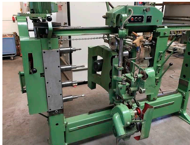
Figure 2. Milling device (Copy Milling Machine COSMA-SKS 7) on which the experiments were performed.
