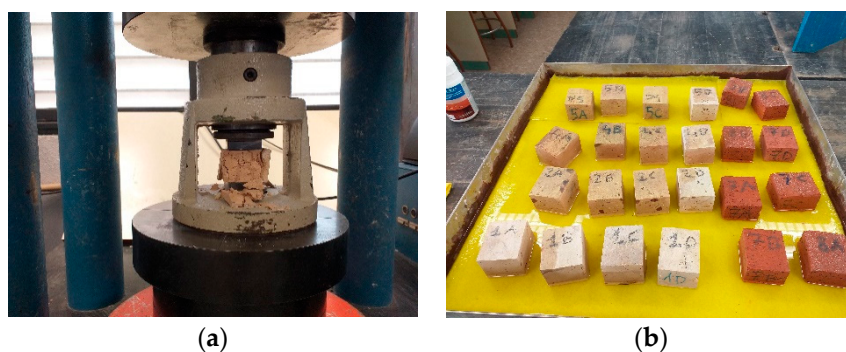
Figure 21. Analyses carried out in the laboratory of the Universitat Politècnica of València: (a) Determination of compressive strength; (b) determination of water absorption by capillarity.
