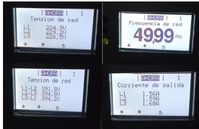
Figure 3. Screenshots showing electrical parameters (voltage, current and frequency).
