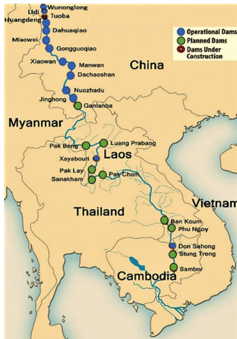
Figure 8. Planned and operational dams across the mainstream of the Mekong River (Recreated: [55]).
