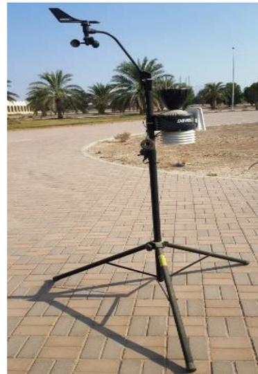
**b****Figure 3.** (a) FLIR E-63900 Infrared Camera. (b) DEVIS Vantage Pro 2 Weather Station.
