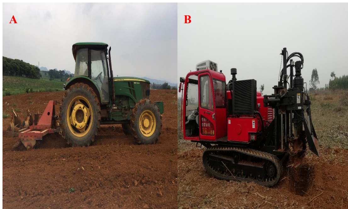
Figure 2. Soil cultivating machinery adopted in the two different tillage practices. The left (A) is conventional tillage (CT, 20 cm), the right (B) is deep vertical rotary tillage (DVRT, 40 cm).
