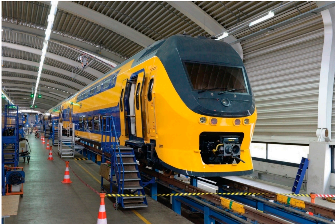
Figure 6. VIRMm1 train during modernization at NSTM, extending its life another 18 years.
