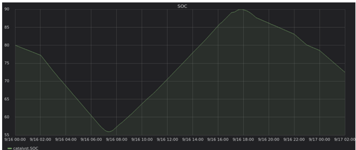
Figure 8. Charging level of the batteries during the test case execution.
