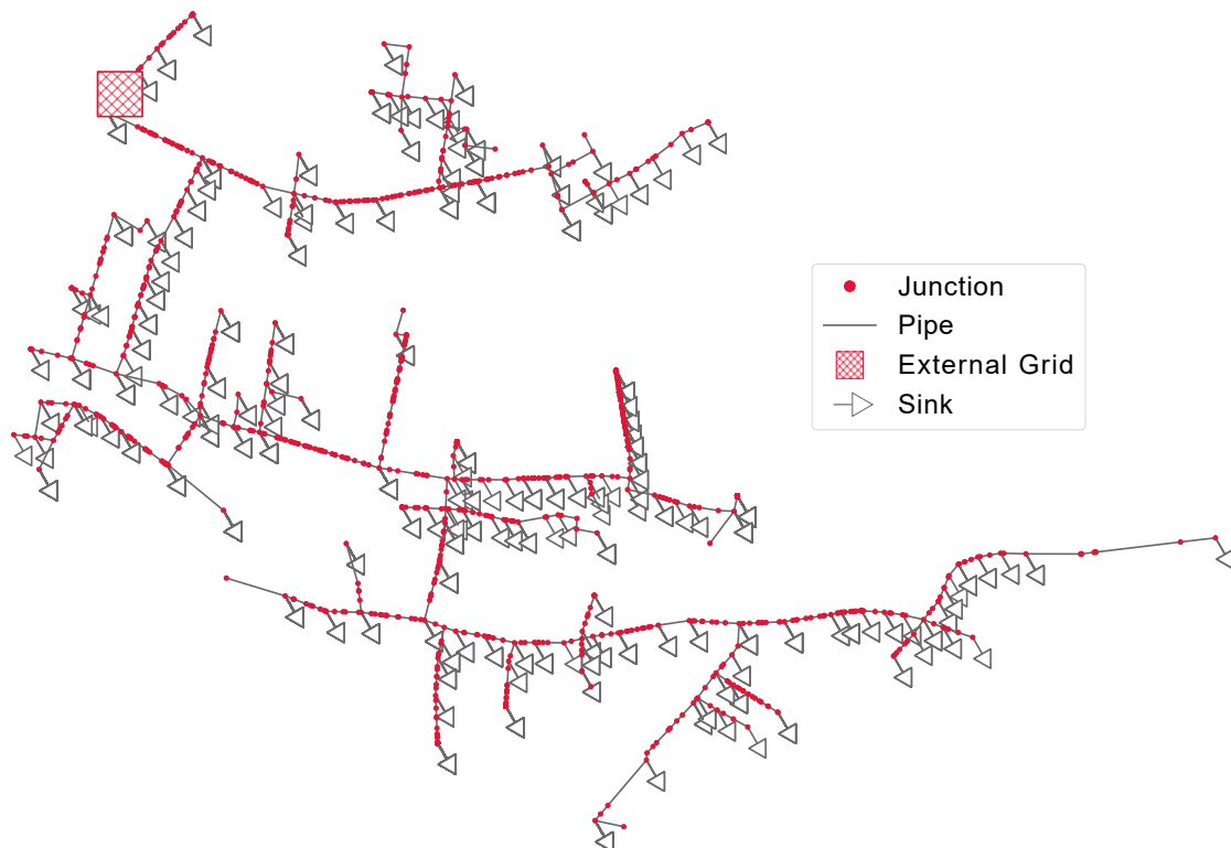
Figure A3. Reduced gas grid used for performance comparison. It comprises 1128 junctions and 1128 pipes, supplies 1506 sinks and is operated at 1 bar.
