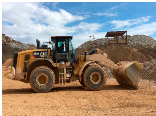
Figure 6. Wheel loader—CAT 972 M.
