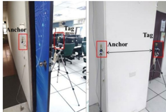
Figure 15. The UWB penetration test. Left: wall thickness = 18 cm. Right: column thickness = 83 cm. The tag and anchor were placed on both sides of the wall, approximately 130 cm above the ground to test the UWB penetration.
