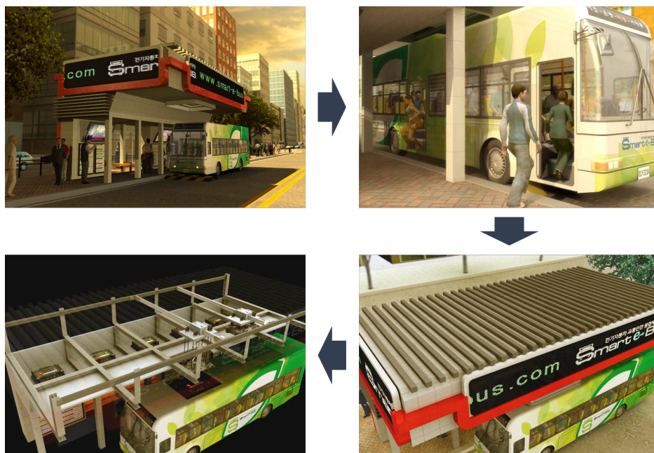
Figure 1. Operational concept of a bus station with Quick Charger Machine (QCM) [13].
