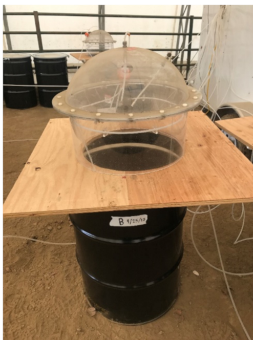
Figure 2. Emission flux chamber covering a 208 L (55 gallons) open-top steel drum containing liquid manure.
