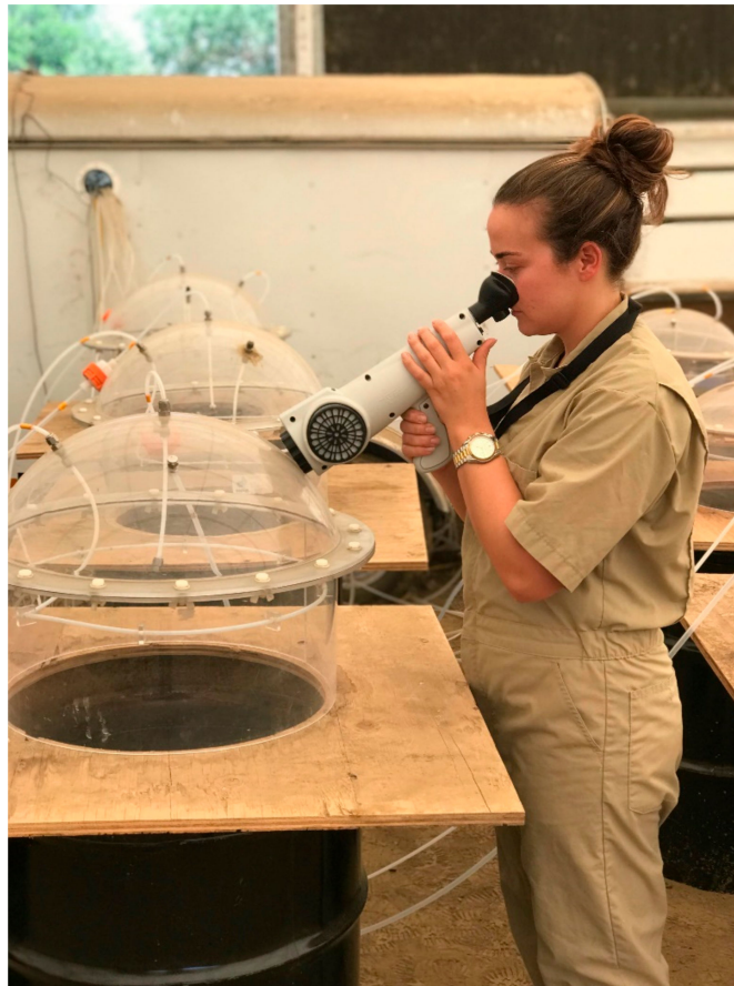
Figure 3. Measurement of odor intensity using the Nasal Ranger approach.
