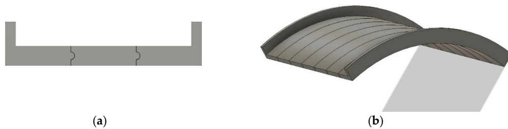
Figure 8. Example of a uni-mold superstructure design to make a modular and adaptable wildlife overpass. This method uses three different FRP structures that can be combined to make versatile wildlife overpasses. (a) Cross-section of three FRP mold proto-types and how they can be connected together to build adaptable bridges. (b) A rendering that shows how adding additional middle sections allows the bridge to be made to any desired width. Figure credit Matthew Bell.
