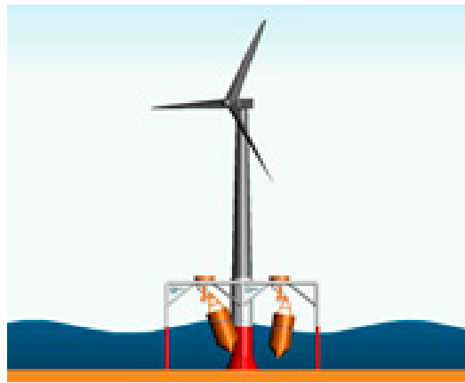
Figure 10. WEGA Hybrid Coupling (Wind turbine + WEC) structure [24].
