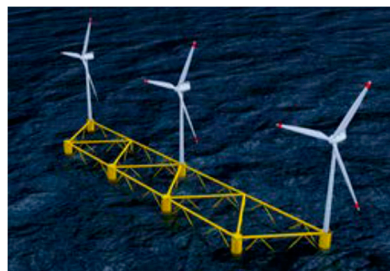
Figure 15. Floating structure that combines wind turbines [24].
