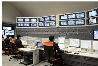
Figure 1. Image of remote human-based monitoring. Source: Yurikamome, Inc. (Tokyo, Japan) provides an automated guideway transit service with unattended train operations. This image is used with permission.
