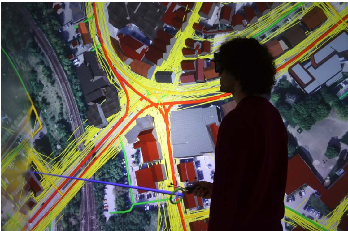
Figure 5. Empirical data set for pedestrian routes and the space syntax model implemented in the urban digital twin. This allows us to compare the movement potential of the street network to real-life uses (photo credited to Dembski, 2018).
