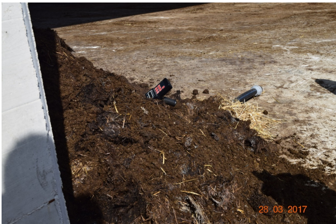
Figure 5. Temperature measurements performed during the composting process by means of a digital probe.
