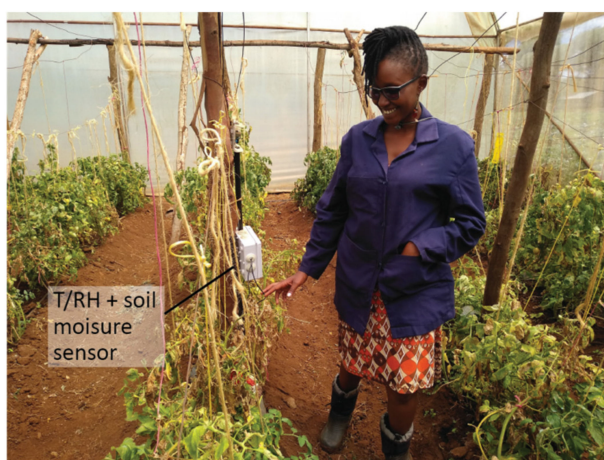
Figure 10. Greenhouse Supervisor inspecting tomatoes and a temperature, humidity, and soil moisture device in a greenhouse at the Dedan Kimathi University of Technology research farm.
