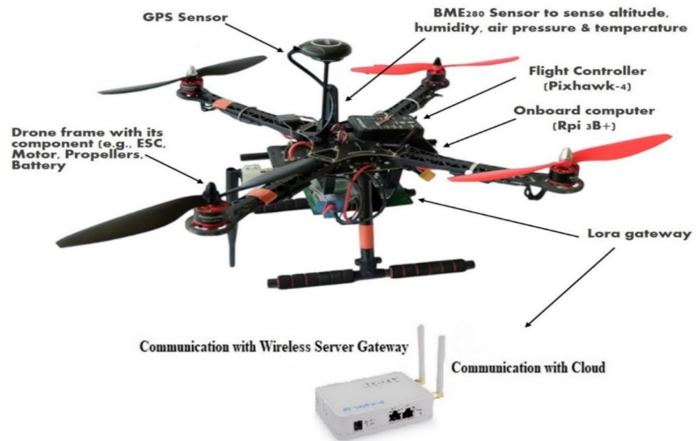
Figure 7. The drone–LoRa gateway.
