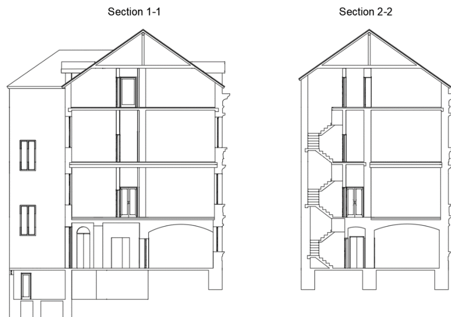
Figure 9. Transversal building sections.
