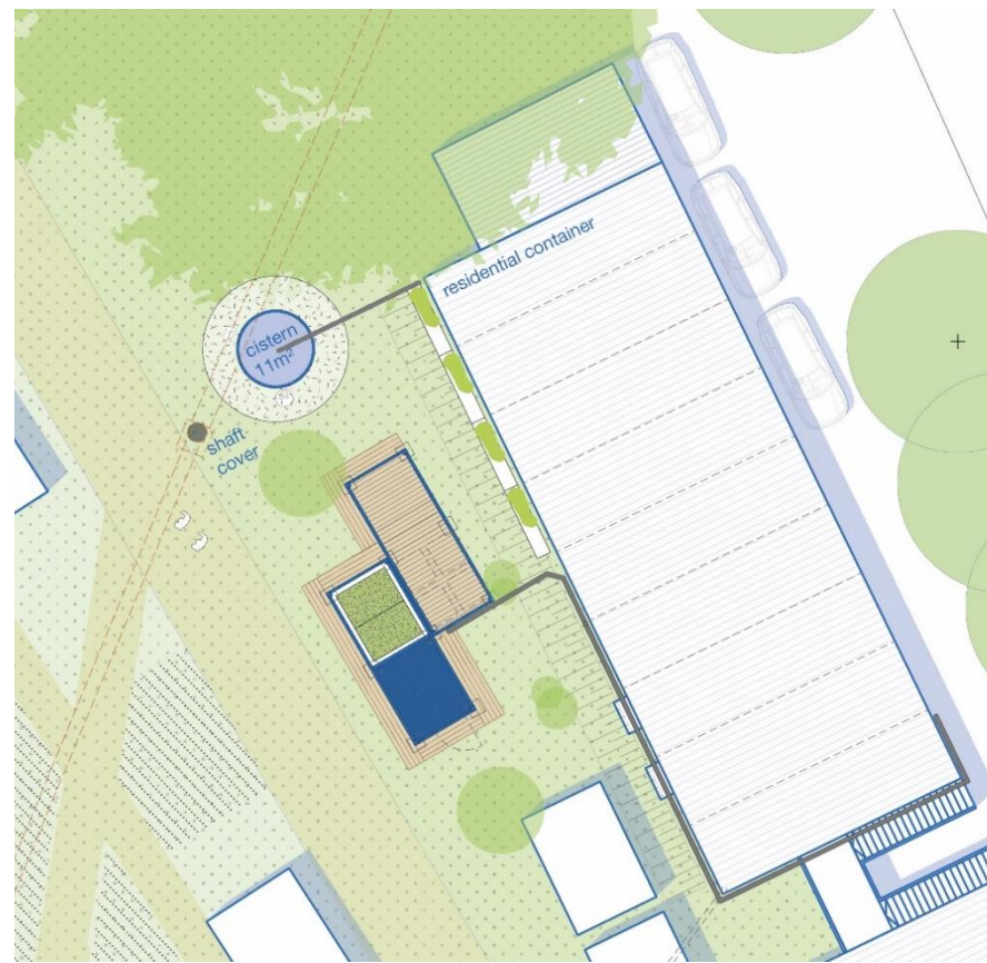
Figure 9. Final design variant V 16 (no scale). The single-storey solution consists of two container frames housing the technical room, the constructed wetland and two terraces, of which one is on top of the grey water storage tanks.
