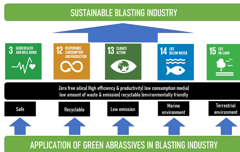
Figure 3. Framework of green abrasives described by six characteristics (1) zero content of free silica, (2) high efficiency and productivity, (3) low consumption media, (4) low amount of waste generation and emission potentials, (5) high recyclability and (6) environmentally friendly in line with sustainable development goals SDG3, SDG12, SDG13, SDG14 and SDG15 for sustainable blasting industry.
