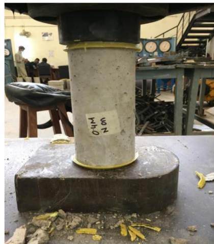
Figure 3. Experimental setup for compression test of SCC and SCGC specimens.
