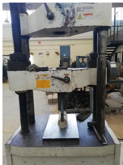
Figure 5. Experimental setup for the split tension test of SCC and SCGC specimens.
