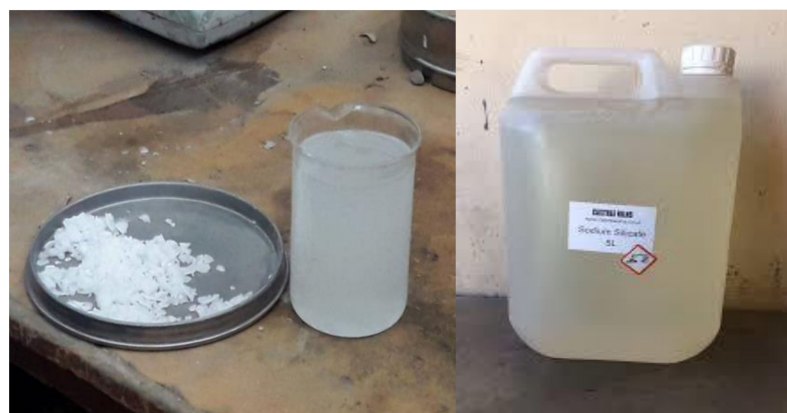
Figure 2. Alkaline Activators NaOH flakes and solution (on left side) and Na 2 SiO 3 solution (on right side).
