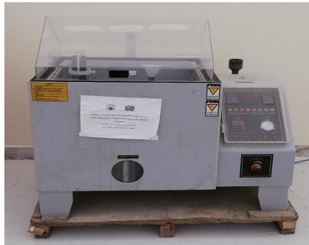
Figure 15. Exposure of specimens in Salt spray test machine.
