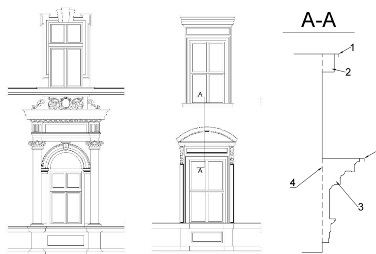
Figure 4. Architectural details of the renovated façade: 1. windowsill; 2. above-window stucco; 3. below-window stucco; and 4. building wall.
