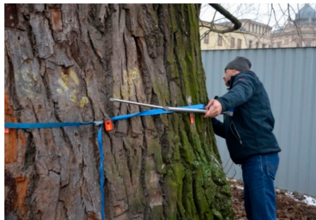
Figure 1. CT scanner sonic located on a tree trunk (W. Durlak, 2021).
