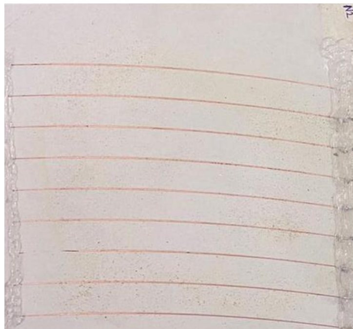
Figure 14. N2 model with 17 mm spacing with 100–300 \mu\text{m} dust distribution.
