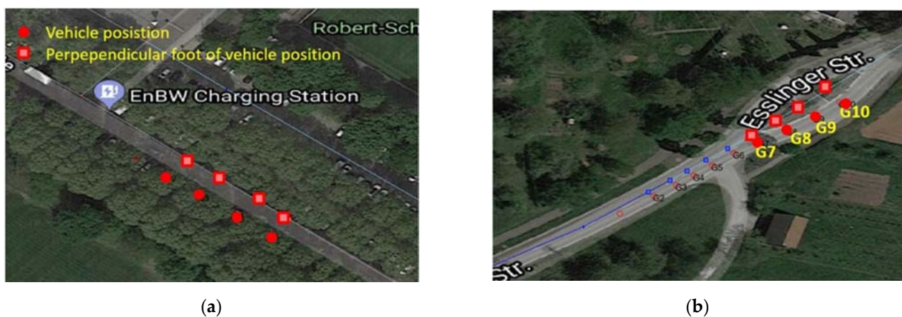
Figure 7. Incorrect off-road estimation due to GNSS inaccuracies (a) and map data inaccuracies (b).
