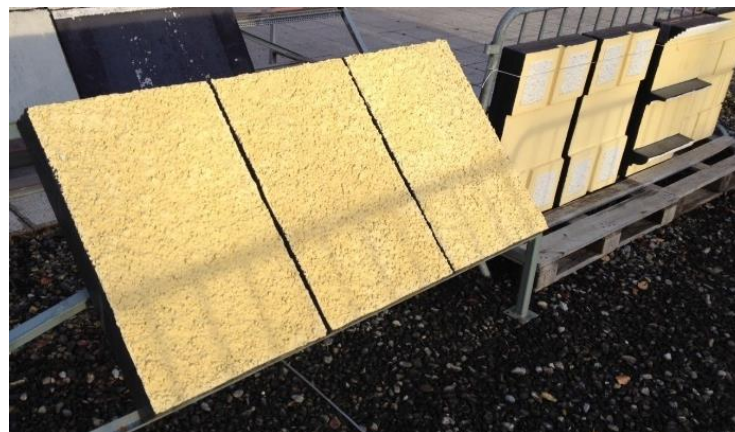
Figure 2. Samples with 6 cm aerogel-based render and 3 different finishing coats weather exposed at an angle of 135° at the R&D of Fixit Group in Röhthis (Austria).
