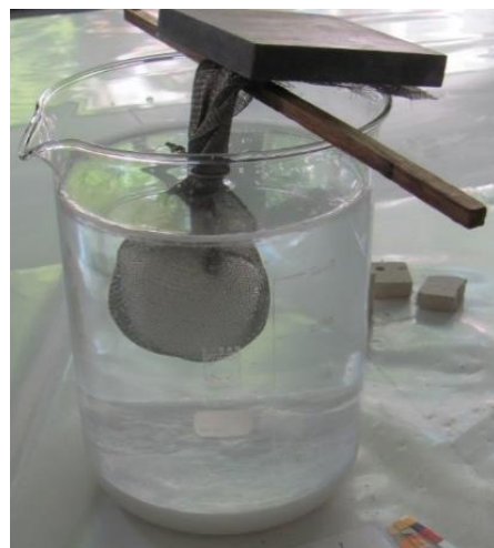
Figure 1. Hydrophobized aerogel granules in a metallic net bag immersed in distilled water.
