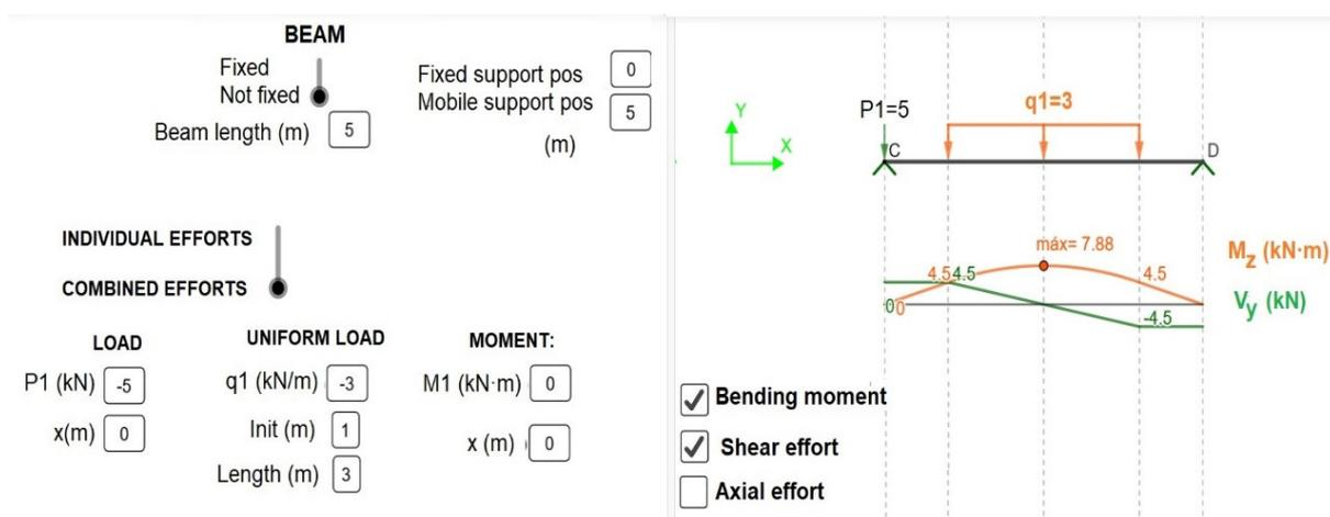
Figure 3. The axial, shear, and bending moment diagrams, highlighting the maximum value.
