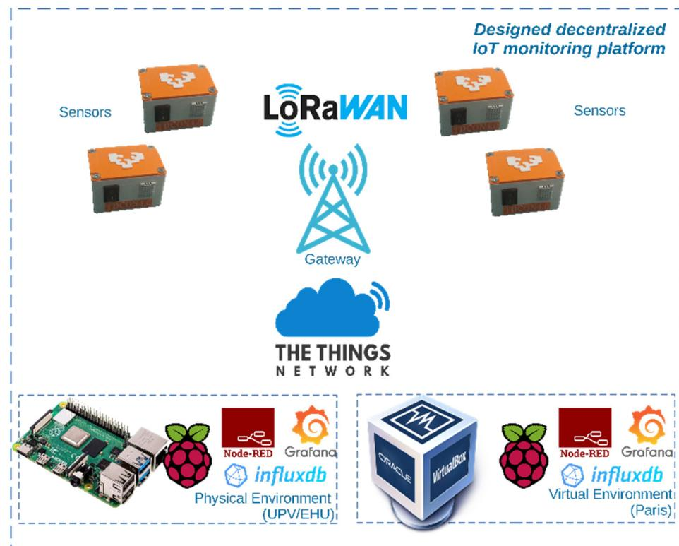
**Figure 4.** Graphical scheme of the implemented RVL methodology.
