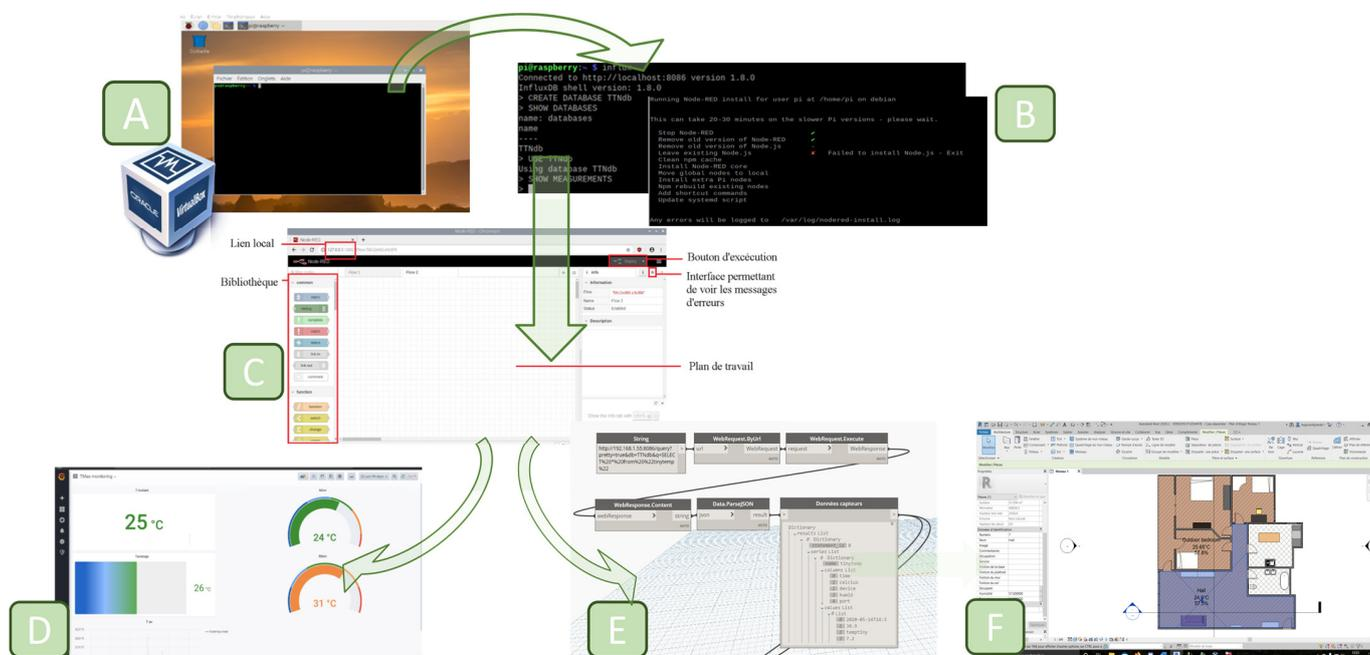
**Figure 7.** Workflow followed by the students under the RVL methodology during the project development. (A): Raspberry Pi OS simulated under VirtualBox, (B): Command-line interface of Raspberry Pi OS, (C): Node-RED environment, (D): designed dashboard in Grafana, (E): developed script in Dynamo, (F): Revit model.
