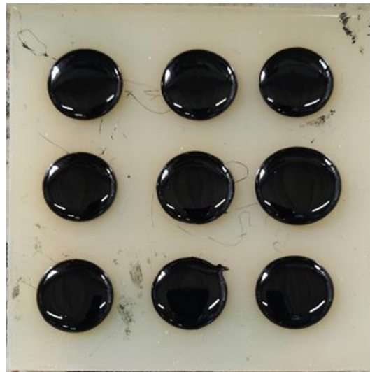
Figure 2. DSR test sample specimens.
