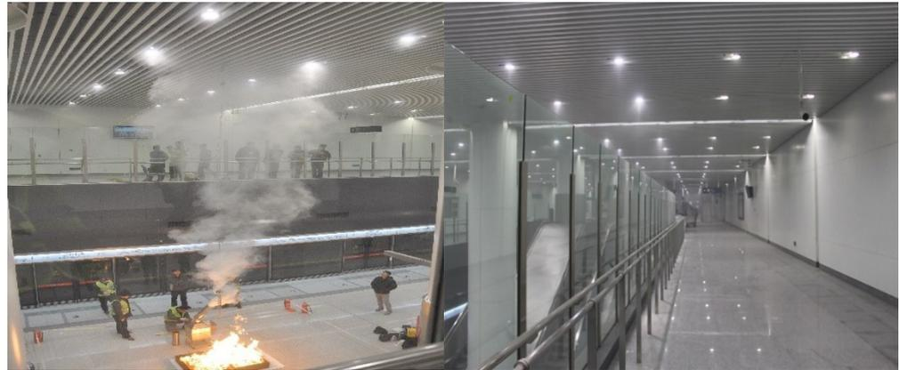
**Figure 16.** The smoke diffusion in Test 2 at station B.
