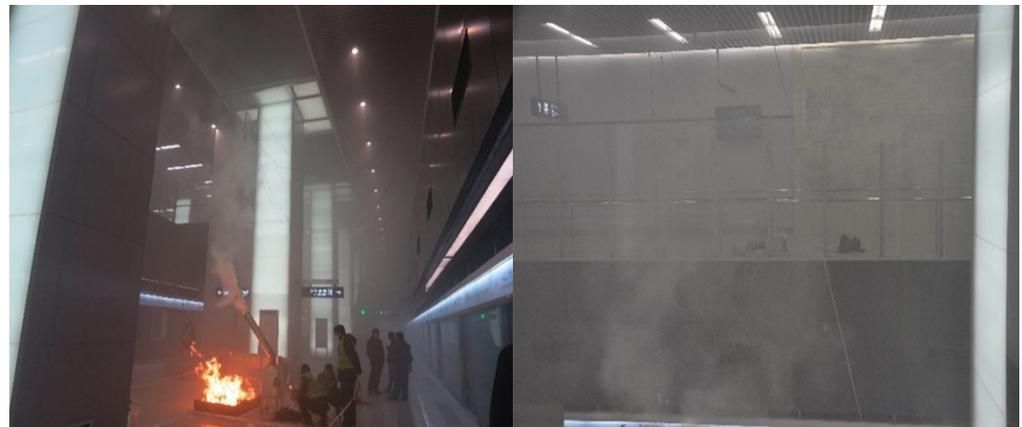
**Figure 17.** The smoke diffusion in Test 3 at station C.
