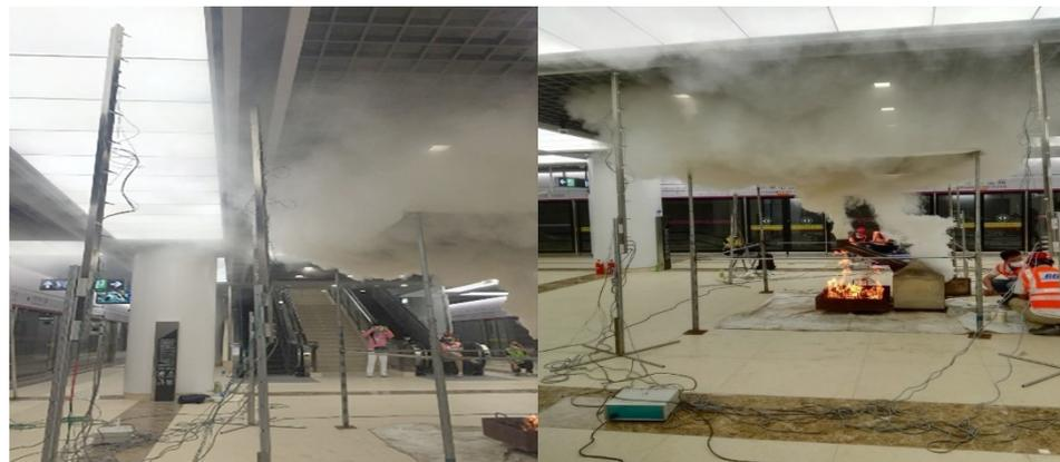
Figure 15. The smoke diffusion in Test 1 at station A.
