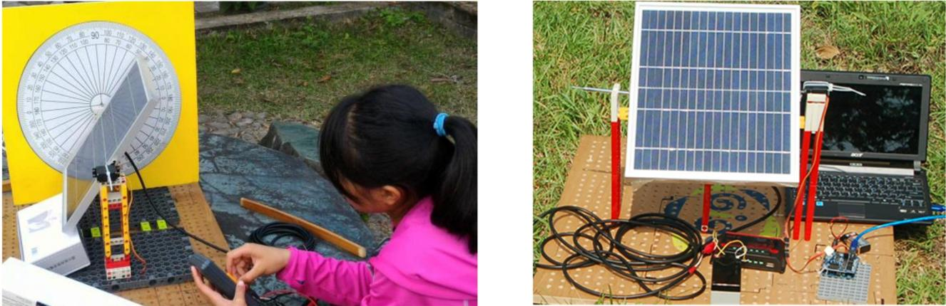
**Figure 7.** Students measured the angle between the solar panel and the sun, using Arduino control to obtain the best storage value ( $S_A-A_3-Y_6$ ).
