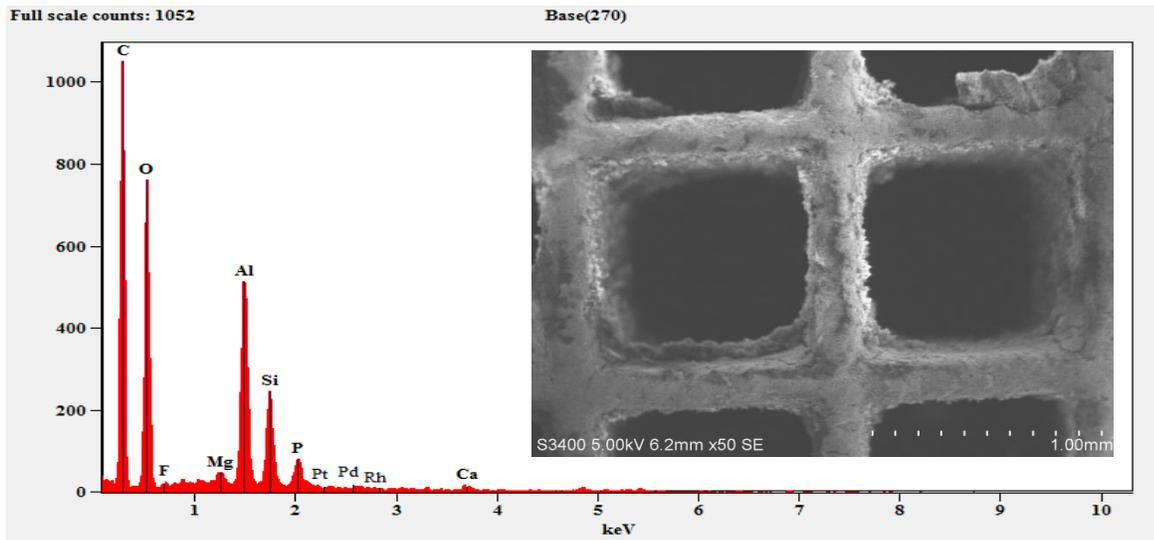
4. EDS peaks of Spent CC Engine side with biodiesel fuel (sample 4), (Figure 6 in the article).
