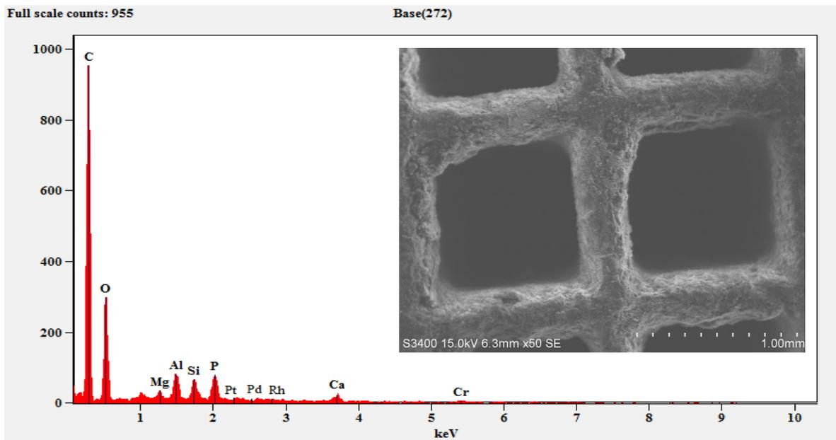
3. EDS peaks of Spent CC exhaust side with diesel fuel (sample 3), (Figure 5 in the article).
