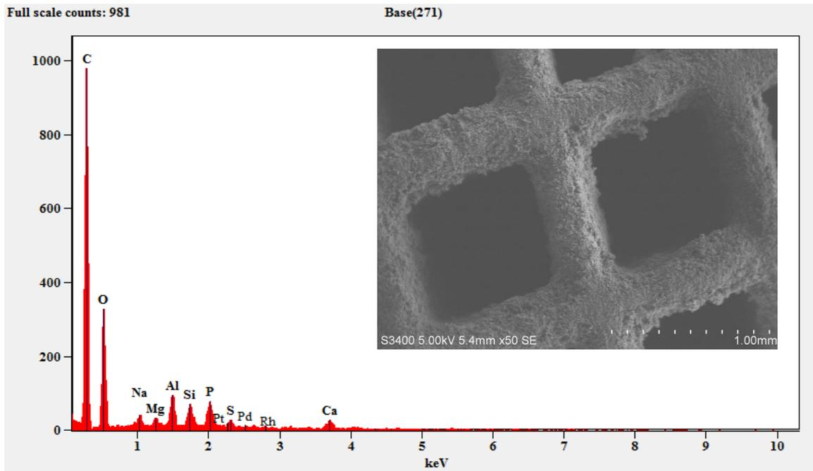
5. EDS peaks of Spent CC exhaust side with biodiesel fuel (sample 5), (Figure 7 in the article).
