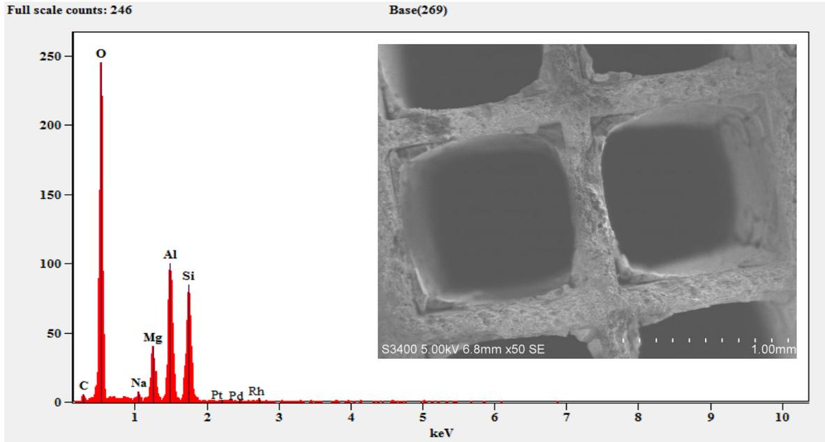
2. EDS peaks of Spent CC Engine side with diesel fuel (sample 2), (Figure 4 in the article).
