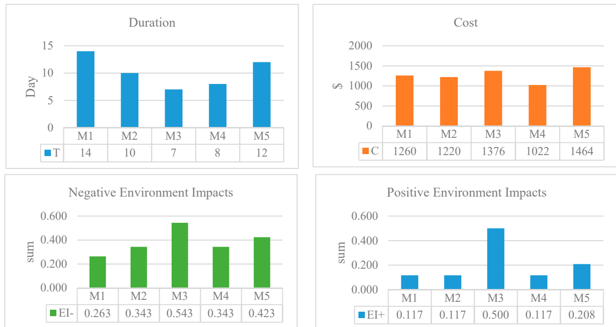
Figure 4. The best execution modes of activity 2 in terms of duration, cost, and positive and negative environmental effects.
