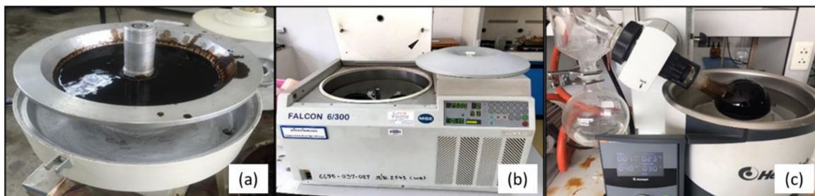
Figure 1. The extraction of aged asphalt binder and aged aggregates from RAP by (a) the extraction unit bowl, (b) the centrifuge, and (c) the rotary evaporator.
