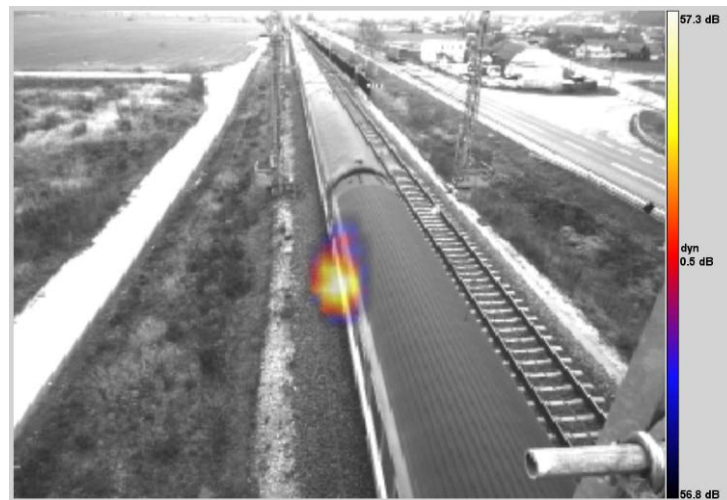
Figure 10. Exterior noise map of the passenger coach—bogie.
