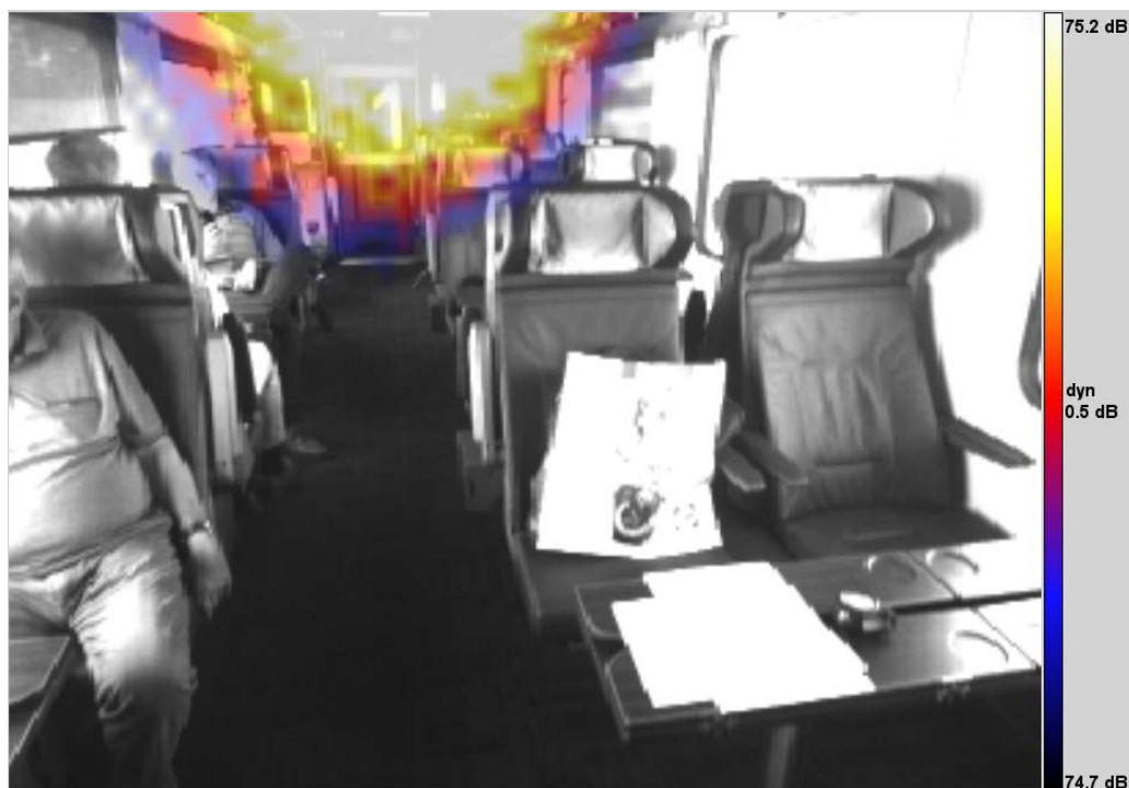
Figure 6. Recording from the acoustic camera—visualization of interior acoustic field.
