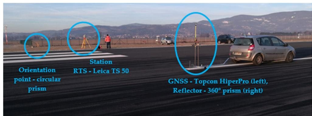
**Figure 2.** Geodetic measuring equipment used in this study.
