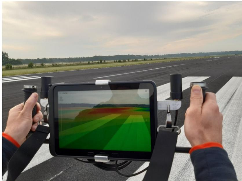
**Figure 9.** Display of surface deformations on the tablet.
