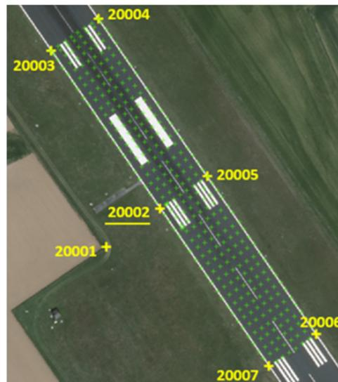
Figure 3. Basic (zero) geodetic net and GRID on the runway.
