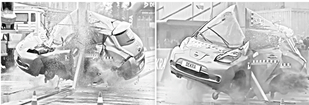
Figure 10. Nissan Leaf pole test by Dekra [44].
