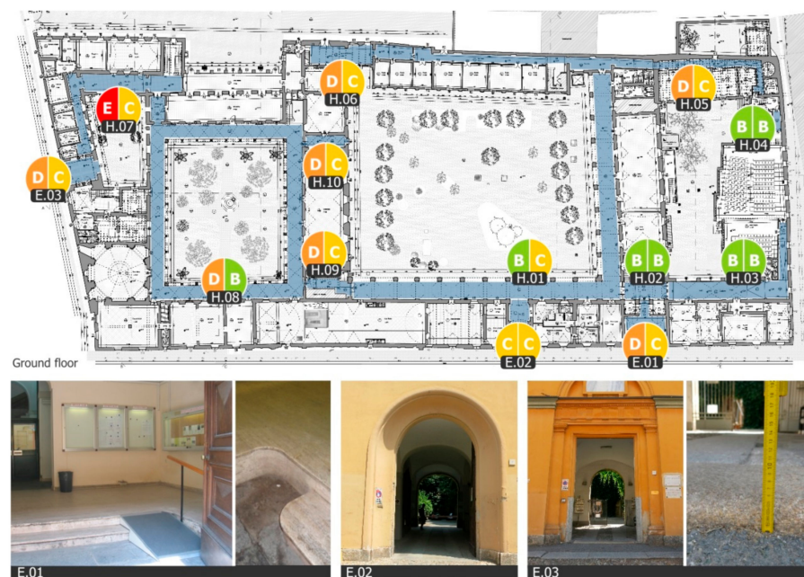
Figure 3. Ground floor of San Felice Palace with the results of the accessibility assessment of entrances (E) and the horizontal connections (H) through the prototype assessment tool A.tool, which provides results into five different levels of accessibility (from A to E) for mobility impairments (left paddles) and visual impairments (right paddles).
