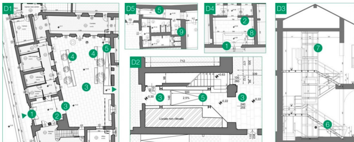
Figure 15. Details (D1, D2, D3, D4, D5) of the design solutions for the ground floor of San Felice Palace: 1. Inclined steel surface with anti-slip treatment; 2. informative-tactile map; 3. paving in stone slabs; 4. stone seats with armrests and space for wheelchairs; 5. new ramp; 6. new metal staircase with double height continuous handrail; 7. new elevator; 8. pantograph platform embedded in the pavement; 9. new accessible toilets.
