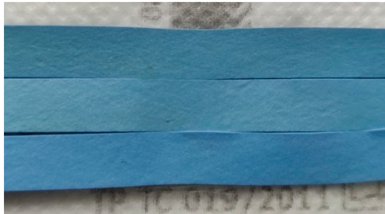
Figure 5. Photo of the elastics showing discolouration after different \text{ClO}_2 sterilisation cycles (Bottom: 0 cycles, middle: 3 cycles, upper: 6 cycles).
