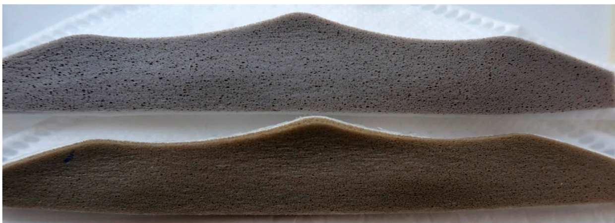
Figure 8. Nose comfort cushion after different \text{ClO}_2 sterilisation cycles (Top: 0 cycles, bottom: 6 cycles).
