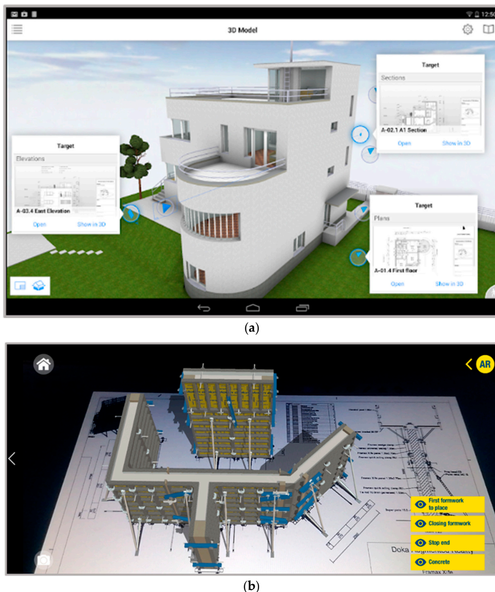
Figure 5. Working environment of visualization of information model: (a) BIMx; (b) Doka AR [58,59].
