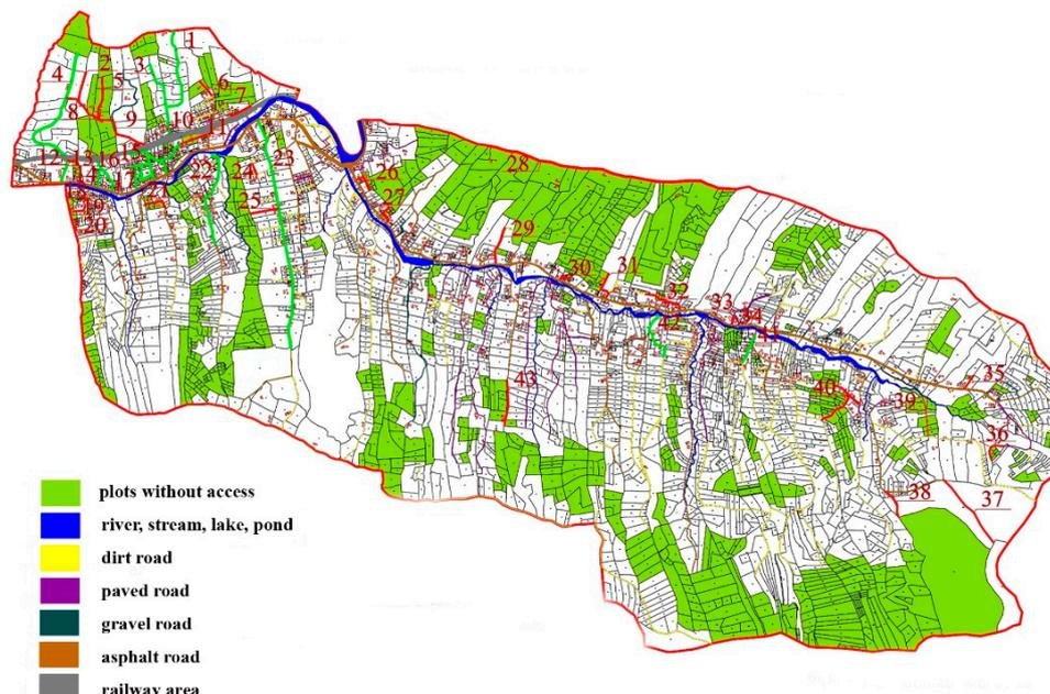
**Figure 9.** Optimal access roads design of Kamionka Wielka (cadastral map, scale of the original: 1:20,000).
