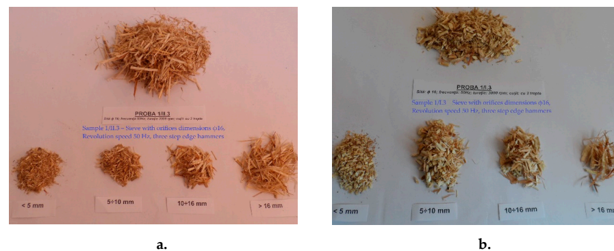
Figure 3. Material subjected to grinding process using a three-step edge hammer and a revolution speed of 50 Hz: (a) Miscanthus Giganteus ; (b) Salix Viminalis .
